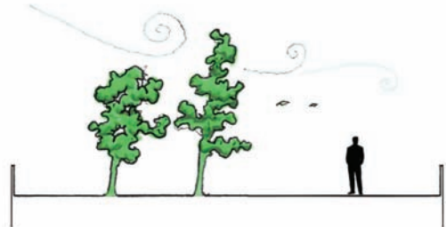
Fig 2: Porous canopy allows wind to pass through, thus reducing wind loads and impacts.
